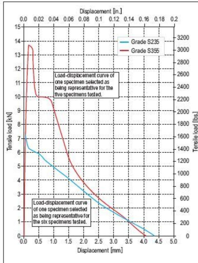
Figure 8. Tension load vs. displacement curve.
