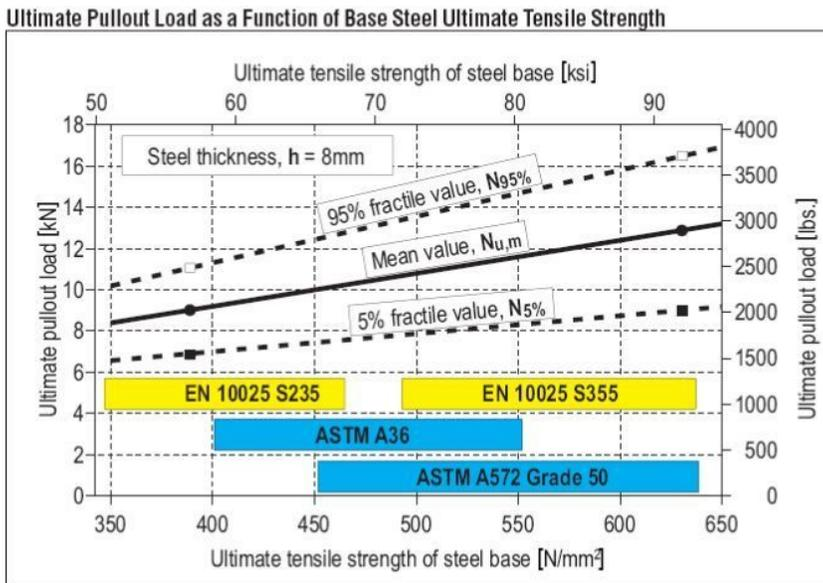
Figure 6. Typical direct axial failure loads for X-BT studs.
