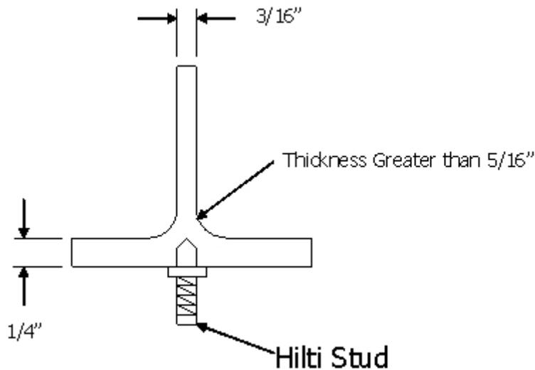
Figure 4. Cross section of stiffener showing stud location on flange coincident with web.
