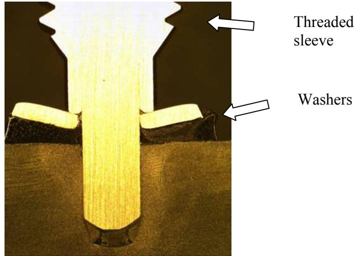
Figure 3. Cross section showing penetration depth/washer compression.
